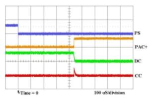
**Case K:** Swap Command Sleep, Falling Edge of PS, PMOD = 1, SWEN = 1, DQ = 0, Cell >  $V_{UV}$ If the device has been swapped into Sleep Mode, SWEN is 1, PMOD is 1, DQ is low, and the cell voltage is above  $V_{UV}$ , then the device entesr Active Mode 450µs after a falling edge on PS. The pins react the same as Case J for the first 2s. However, because PMOD is 1 and DQ is low, the device reenters Sleep Mode after 2s.
