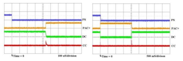
**Case L:** Swap Command Sleep, Falling Edge of PS, PMOD = 1, SWEN = 1, DQ = 1, Cell >  $V_{UV}$ If the device has been swapped into Sleep Mode, SWEN is 1, PMOD is 1, DQ is high, and the cell voltage is above  $V_{UV}$ , then the device enters Active Mode 450µs after a falling edge on PS. The pins react the same as Case J.
